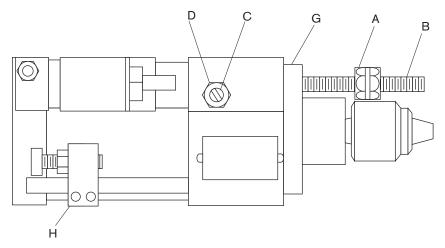
The Hypneumat Hydra-Brake is a self contained hydraulic cylinder with an adjustable feed rate through a Needle Valve. The Hydra-Brake is mechanically actuated by the Quill Clamp ("G") of the Hypneumat Stroke Control Assembly. The forward stroke of the Hydra-Brake is controlled through the needle valve ("C"). The return stroke of the Hydra-Brake is not restricted.
