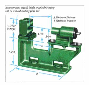
No. 22-X (22HC99) Vertical Hand Index & Horizontal Clamping Fixture for holding piece parts while drilling or tapping a series of holes at angles to each other. Hand Indexing. (22HCL99 - extra long base / 22NX799 release valve
