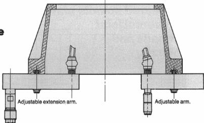
Standard fixed position plate showing a collet type spindle assembly.
